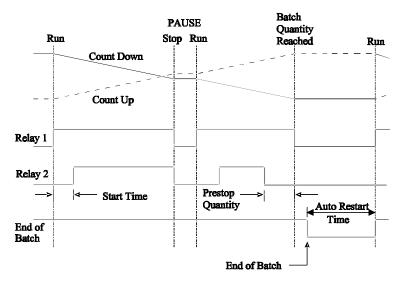
The Batch Controller can be configured to either count up from zero on each batch or to count down from the preset batch quantity.
